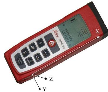
The main result of this note is that a well-calibrated DistoX is accurate in measuring directions, ie, the measured values of azimuth and inclination agree (within the measurement uncertainties) with the real azimuth and inclination.
